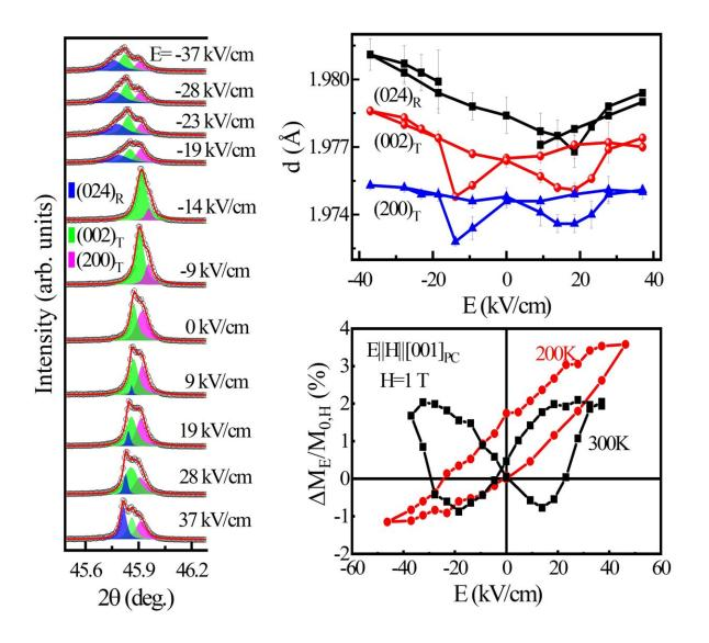
High resolution X-ray diffraction patterns at in-situ applied electric fields, corresponding variation of lattice spaces with applied electric fields, and
