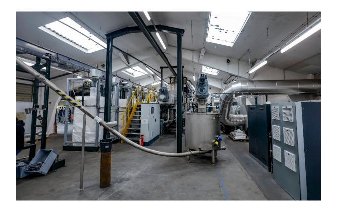
Biochar is produced by heating cocoa bean husks in an oxygen-free room to 600 degrees Celsius (1112 Fahrenheit).
