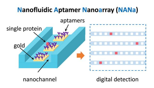
Schematic illustration of the NANa principle for stochastically capturing and digitally detecting single proteins. Credit: Yan Xu, Osaka Metropolitan University
