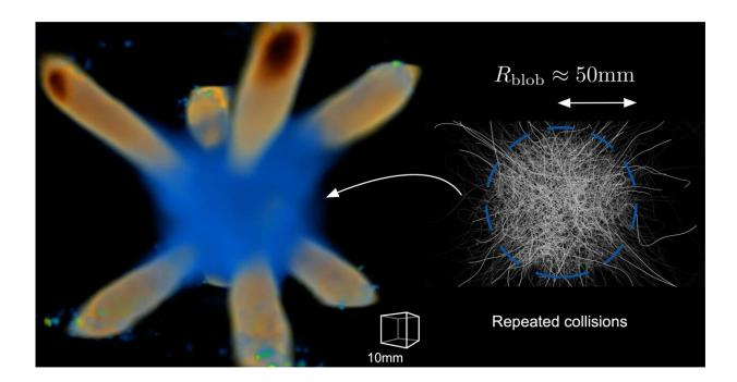
Repeated collision of eight vortex rings forms an isolated blob of turbulence. (Left) The decomposition of the blob energy into mean flow (yellow) and fluctuating (blue) parts illustrates the formation of confined turbulence. (Right) Highly irregular trajectories of tracer particles are observed inside the turbulent blob. Credit: Matsuzawa et al
