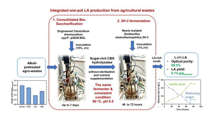
Schematic representation of the integrated LA production process from agrowastes. Credit: LIU Yajun
