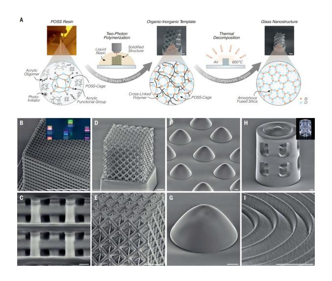
Fabrication of high-quality fused silica nanostructures from an acrylate-functionalized POSS resin. (A) Schematic synthesis through TPP 3D printing
