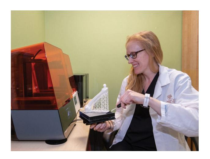
Barnes removes a newly printed 3D model and its scaffolding (connecting the printed bone to the platform) from the printer's build platform (black). Once removed from the platform, the bone model is detached from the scaffolding. Credit: Texas A&M University School of Veterinary Medicine & Biomedical
