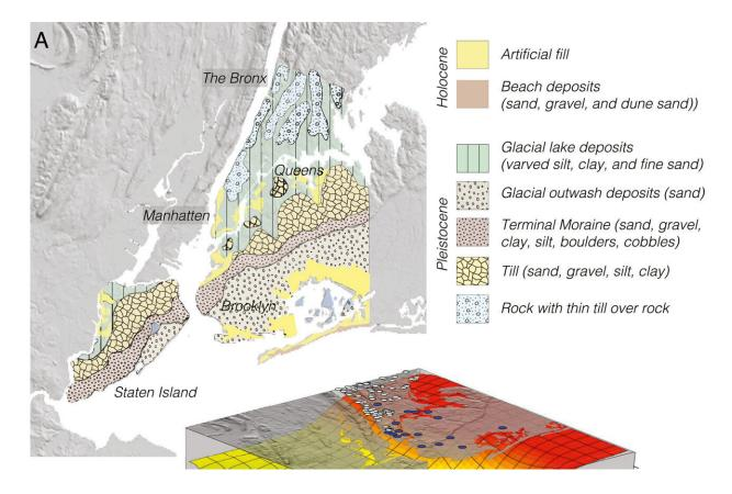
(a) Surface geology map of New York City after Nikolaou et al. (2001) and Tamaro et al. (2000). (b) Soil-bedrock interface interpolated from well data (Nikolaou, 2004) and outcrop observations. Blue dots represent well locations and white dots are bedrock outcrops. Credit: *Earth's Future* (2023). DOI: 10.1029/2022EF003465
