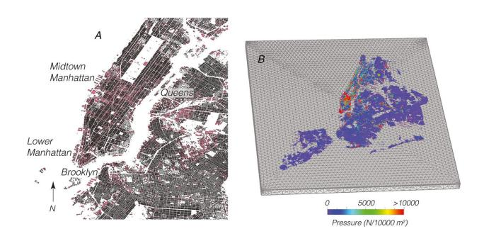
(a) Excerpt from building base outline database for New York City showing parts of Manhattan, Queens, and Brooklyn. Base outlines and height data were used to calculate total building floor areas, which combined with live and dead load values yields a building's mass. (b) The combined building load profile distributed in 100 m-by-100 m cells is shown superposed on the finite element model used to calculate subsidence. Credit: *Earth's Future* (2023). DOI: 10.1029/2022EF003465
