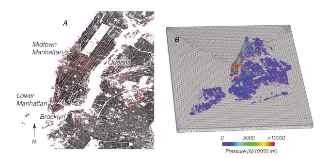
(a) Excerpt from building base outline database for New York City showing parts of Manhattan, Queens, and Brooklyn. Base outlines and height data were used to calculate total building floor areas, which combined with live and dead load values yields a building's mass. (b) The combined building load profile distributed in 100 m-by-100 m cells is shown superposed on the finite element model used to calculate subsidence. Credit: *Earth's Future* (2023). DOI: 10.1029/2022EF003465
