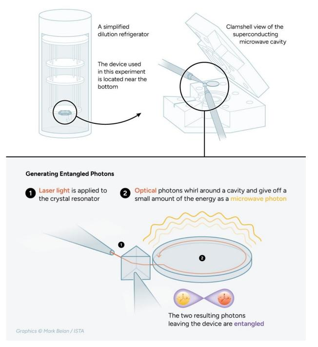
The experimental setup with the dilution refrigerator, the superconducting
