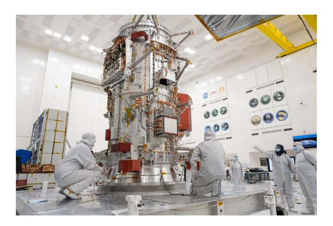
Engineers and technicians work on the towering main body of NASA's Europa Clipper spacecraft at the agency's Jet Propulsion Laboratory. A new video series lifts the curtain on the clean room and shows audiences what goes into building space missions. Credit: NASA/JPL-Caltech
