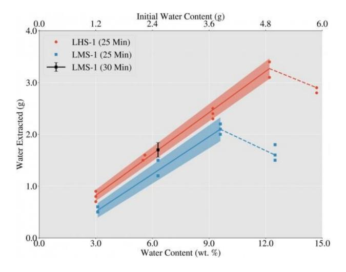
The fraction of water extracted by microwaves. Credit: Cole, et al
