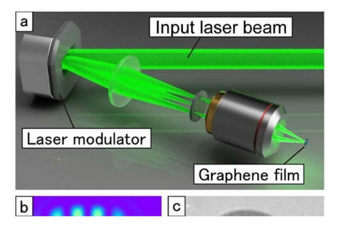
(a) Schematic of the laser processing system. (b) Formation of 32 laser spots on the graphene film. (c) Image of a graphene film that has been multi-point hole-drilled. ©Yuuki Uesugi et al.
