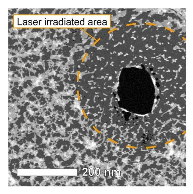
Image of laser-processed graphene film observed by scanning transmission electron microscopy. The black areas indicate through-holes. The white objects indicate surface contaminants. ©Yuuki Uesugi et al.
