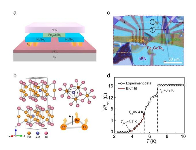
S/F/S device architecture and temperature-dependent resistivity. **a** Schematic illustration of a S/F/S lateral Josephson junction. **b** Schematic diagram of the atomic structure of  $Fe_3GeTe_2$ , where showing noncoplanar spin textures with a fictitious field of *h* in a frustrated triangular lattices. **c** Optical image of the
