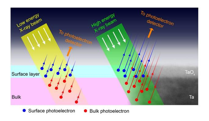
Tantalum oxide (TaO<sub>x</sub>) being characterized using x-ray photoelectron spectroscopy. Credit: Brookhaven National Laboratory
