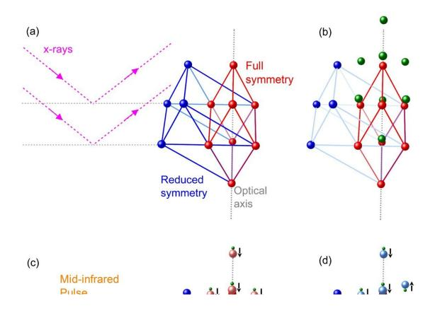
Magenta dashed lines with arrows illustrate diffraction of hard femtosecond x-ray pulses off the lattice planes of the Bi crystal. Red balls connected by red lines: unit cell of an unexcited bismuth crystal containing two Bi atoms with one atom at its origin. The second atom is shown as green balls in panel (b) and is indicated as small balls in panels (c) and (d). Blue balls connected by blue lines: unit cell of the photo-excited crystal with reduced symmetry containing four Bi
