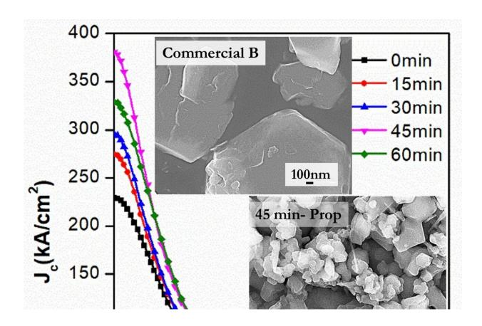
Scientists at SIT in Japan produced high-performance MgB2 by ultrasonicating boron (B) in 2-propanol for varying durations. The inset displays high magnification FE-SEM images of B particles obtained after 0 and 45 minutes, respectively, with the latter showing 20-50 nm refined grains. Credit: Muralidhar Miryala from Shibaura Institute of Technology (SIT), Japan
