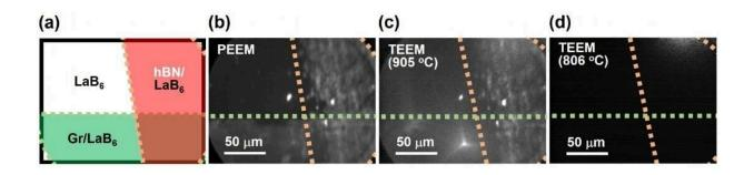
Photoemission electron microscopy (PEEM) and thermal electron emission microscopy (TEEM) images of  $LaB_6$  surface coated with graphene (Gr) and hBN. Bright areas in the images indicate a large number of emitted electrons. Credit: Hisato Yamaguchi et al
