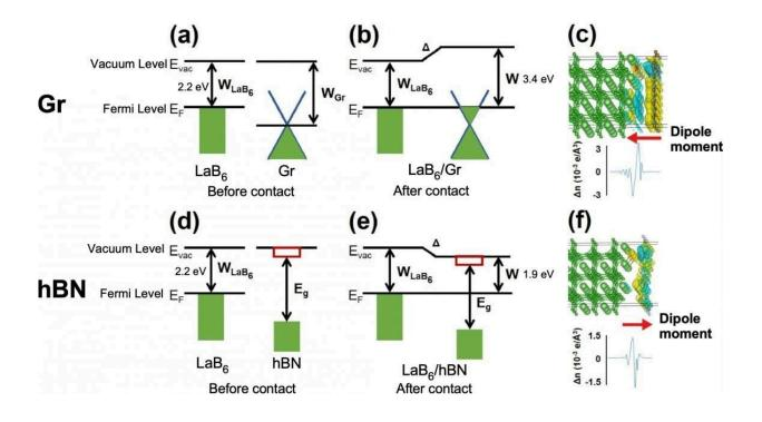
A schematic diagram of the work function modulation mechanism by graphene and hBN coating. When  $LaB_6$  and coating material come into contact by coating, their Fermi levels (EF) become equal. In the case of coating  $LaB_6$  with graphene ((a), (b)), the work function W after graphene coating is larger than the original
