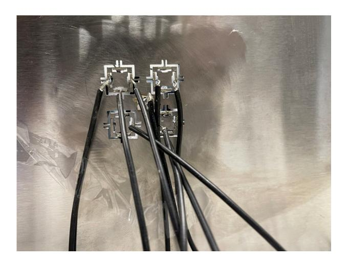
The prototype metamaterial uses electrical signals transported by these black wires to control both the direction and intensity of energy waves passing through a solid material. Credit: University of Missouri
