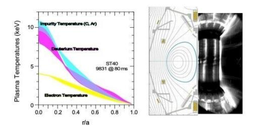
Results from TRANSP analysis of high temperature ST40 discharge (left) and equilibrium reconstruction and camera image of high temperature ST40 discharge (right). Credit: Princeton Plasma Physics Laboratory, Princeton University (left) and Tokamak Energy Ltd. (right).
