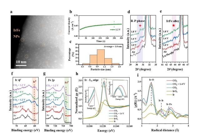
(a) Dark field-STEM image of the SFIrM catalyst after (b) reconstruction at 1.2 V and (c) the corresponding diameter distribution of exsolved IrFe alloy NPs. (d-e) In situ XRD patterns at 29-33° and 41-47°. (f-g) In situ NAP-XPS spectra of Ir 4f and Fe 2p. (h-i) In situ Ir L3-edge XANES spectra and the corresponding Fourier transformed EXAFS spectra. Credit: Science China Press
