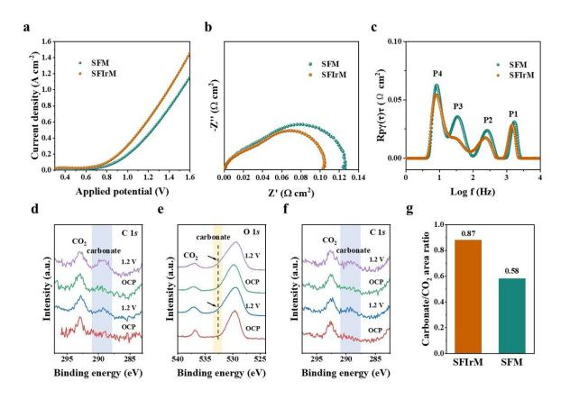
(a) LSV curves of the electrolysis cells with SFM and SFIrM cathodes. (b) EIS plots and (c) corresponding DRT analysis at 1.4 V. (d-e) In situ NAP-XPS spectra of C 1s and O 1s of the SFIrM cathode, and (f) in situ NAP-XPS spectra of C 1s of the SFM cathode. (g) The area ratio of carbonate/CO2 deconvoluted from (d) and (f), respectively. Credit: Science China Press
