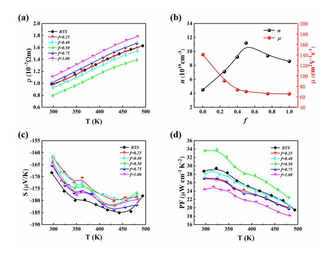
Dependence of (a) electrical resistivity; (b) hall concentration and mobility; (c) thermopower; (d) power factor; of BTS/fwt%MnSb<sub>2</sub>Se<sub>4</sub> (f=0, 0.25, 0.40, 0.50, 0.75 and 1.00) samples with temperature. Credit: Chen Tao
