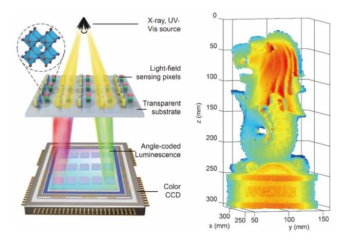
Design (left) and output (right) of 3D light-field sensor. The designed device (left) encodes the light field as color output. Patterned perovskite nanocrystals arrays convert different directions of light into different colors, which can be detected by a color charge-coupled device camera. The right image shows a reconstructed 3D depth image of a Merlion model produced by the camera. Credit: Yi Luying
