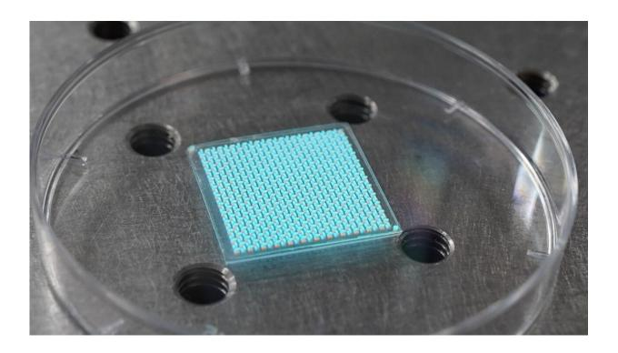
A large scale angle-sensing structure comprising nanocrystal phospors, a key component of the sensor, illuminated under ultraviolet light. Three light emitting phosphors that produce red, green and blue light are arranged in a pattern to capture detailed angular information which is then used for 3D image construction. The team is looking into using other materials for the structure too. Credit: National University of Singapore
