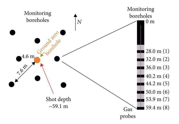
Map view (left) and cross-section (right) of the GZ borehole and 8 monitoring boreholes with locations of gas samplers. Yellow zones are zones of sand and epoxy which hold the gas sniffers. Gray zones are grout. Not to scale, grout layers are 5-7 times the height of the sand/epoxy layers. Credit: *Geofluids* (2021). DOI: 10.1155/2021/6697819
