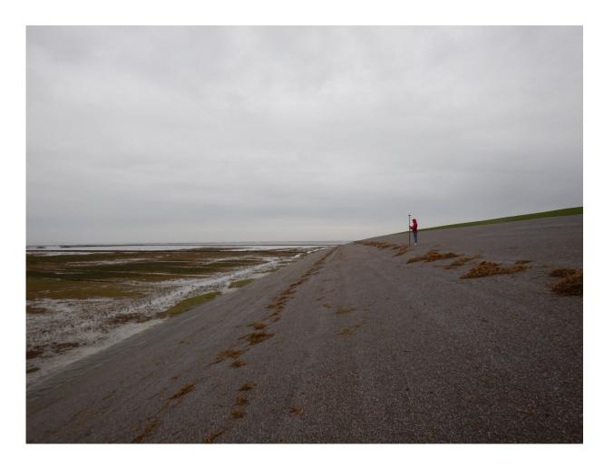
This image shows how the tide mark on a dike is measured after a storm. Credit: B. Marin-Diaz, University of Groningen
