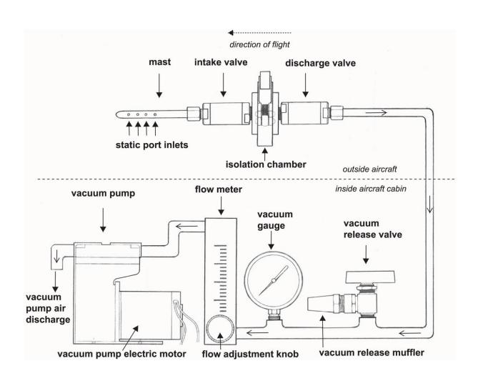
A schematic drawing of our high-integrity probe and supporting system for air eDNA sampling. Credit: *PeerJ* (2023). DOI: 10.7717/peerj.15171
