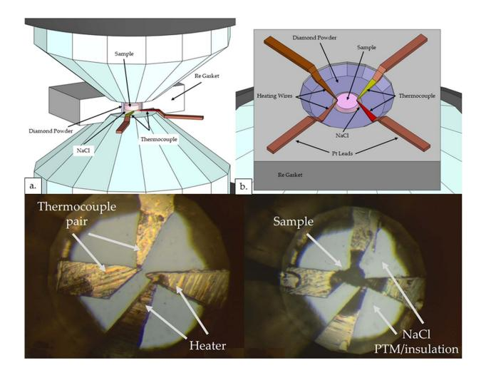
The heat-capacity setup [from the March 2023 article published by the University of Rochester team]. Top, schematic rendering of the new a.c calorimetry technique (not to scale). The sample is surrounded by a NaCl insert with a heater and thermocouple making contact with the sample. a, View of the
