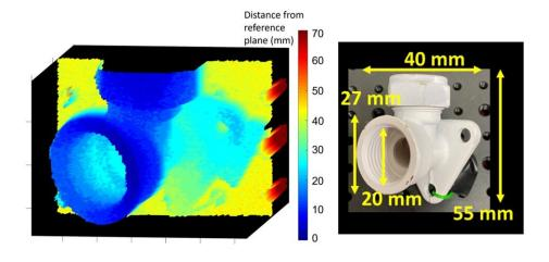
Researchers developed a lidar system that uses quantum detection technology that can capture 3D images while submerged underwater. They demonstrated the system by using it to capture a 3D image (left) of a pipe (right). The scan was obtained in low scattering conditions with the single-photon system submerged in a tank. Credit: Aurora Maccarone, Heriot-Watt University
