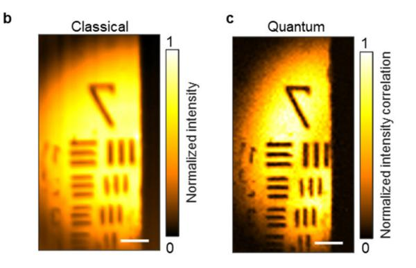
Images produced by standard microscopy and quantum microscopy. Credit: Caltech
