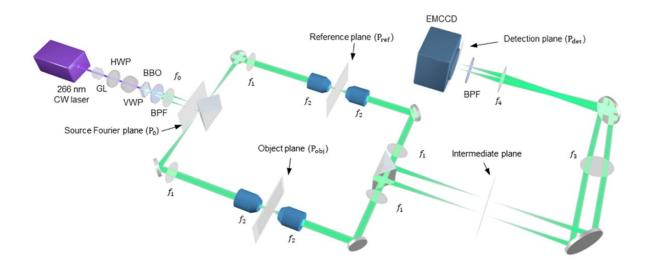
A diagram of the quantum microscopy by coincidence apparatus. Credit: Caltech
