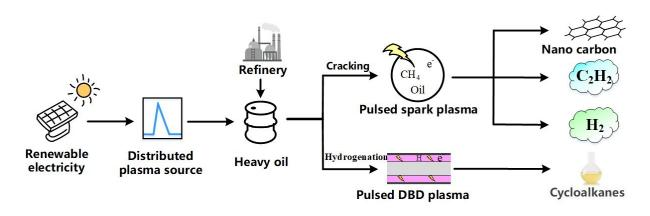
Fig. 2 Application scenario of plasma-enabled heavy oil processing. Credit: IEE
