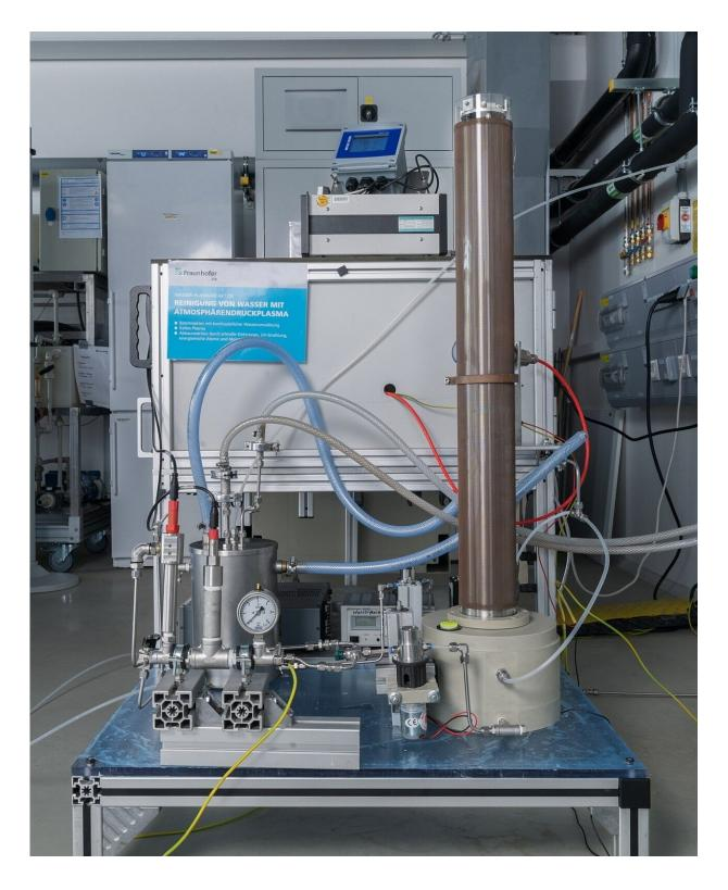
Pilot plant for the elimination of PFAS. Following the initial success of the trials, the technology is now to be optimized and scaled up for practical applications on an industrial scale. Credit: Fraunhofer-Gesellschaft
