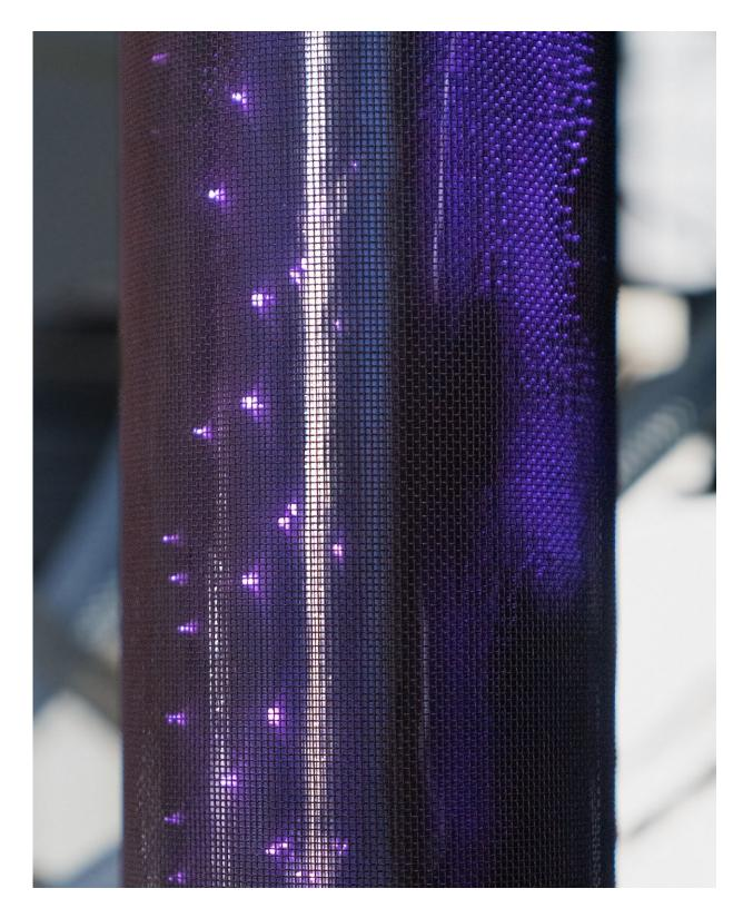
The plasma atmosphere is clearly visible in the reactor through the characteristic glow and flashes of light. Credit: Fraunhofer-Gesellschaft
