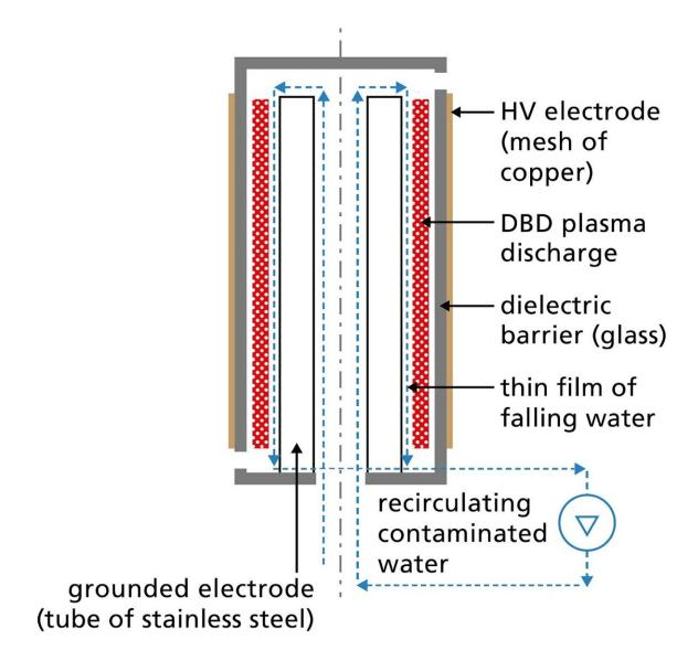
Plasma reactor: Plasma is created by applying voltage to the copper electrode. Contaminated water is pumped upwards and flows back down through a gap in the plasma discharge zone, attacking the PFAS in the process. Credit: Fraunhofer-Gesellschaft
