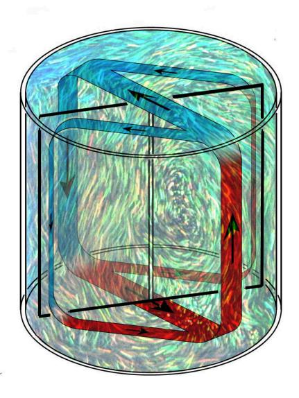
A recent experimental study, inspired by the super-rotation of the Earth's solid core, shows when turbulence flows contained in a cylinder interact with a free body a surprisingly smooth rotation is observed. The red (warm) and blue (cold) ribbons represent water flows. Credit: Kaizhe Wang and Jun Zhang.
