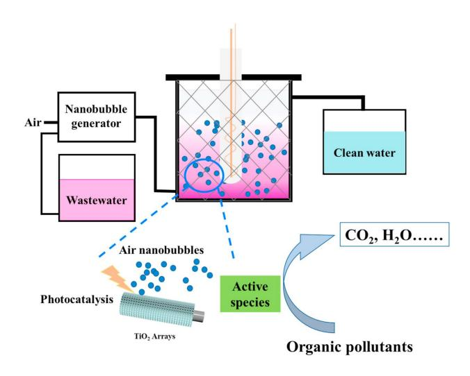
The cylindrical reactor was made of stainless steel with a diameter of 210 mm and a height of 210 mm. The Ti meshes (100 mm in length, 100 mm in width, and 0.5 mm in thickness) coated with  ${\rm TiO_2}$  nanotubes Arrays were fixed inside the reactor. A 100 W high-pressure mercury lamp (HPML) was placed inside the quartz tube. In addition, the inlet and outlet were designed on the left and right
