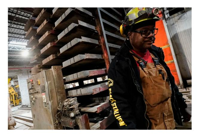
A stack of concrete blocks created with liquid carbon dioxide as an ingredient is pulled from a curing kiln at the Glenwood Mason Supply Company, Tuesday, April 18, 2023, in the Brooklyn borough of New York. New York is forcing buildings to clean up, and several are experimenting with capturing carbon dioxide, cooling it into a liquid and mixing it into concrete where it turns into a mineral. Credit: AP Photo/John Minchillo
