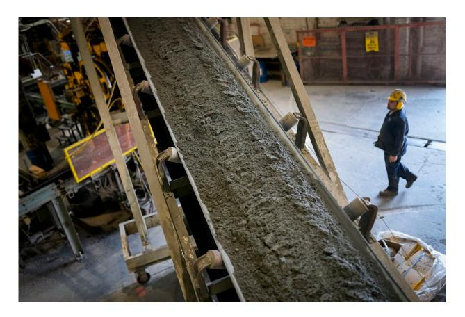
Fresh concrete is fed via a conveyor belt into a forming machine, producing blocks designed with liquid carbon dioxide as an ingredient at the Glenwood Mason Supply Company, Tuesday, April 18, 2023, in the Brooklyn borough of New York. New York is forcing buildings to clean up, and several are experimenting with capturing the carbon dioxide, cooling it into a liquid and mixing it into concrete where it turns into a mineral. Credit: AP Photo/John Minchillo
