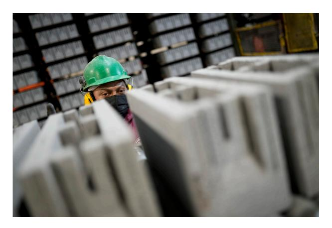
Workers monitor a production line of concrete blocks, made with liquid carbon dioxide as an ingredient, at the Glenwood Mason Supply Company, Tuesday, April 18, 2023, in the Brooklyn borough of New York. New York is forcing buildings to clean up, and several are experimenting with capturing carbon dioxide, cooling it into a liquid and mixing it into concrete where it turns into a mineral. Credit: AP Photo/John Minchillo
