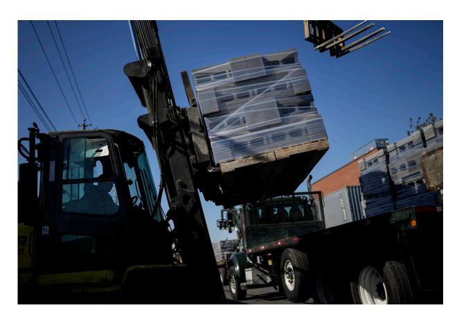
A forklift operates a load of concrete blocks, made with liquid carbon dioxide as an ingredient, onto trucks at the Glenwood Mason Supply Company, Tuesday, April 18, 2023, in the Brooklyn borough of New York. New York is forcing buildings to clean up, and several are experimenting with capturing carbon dioxide, cooling it into a liquid and mixing it into concrete where it turns into a mineral. Credit: AP Photo/John Minchillo
