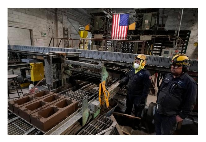
Workers monitor a production line of concrete blocks created with liquid carbon dioxide as an ingredient at the Glenwood Mason Supply Company, Tuesday, April 18, 2023, in the Brooklyn borough of New York. New York is forcing buildings to clean up, and several are experimenting with capturing carbon dioxide, cooling it into a liquid and mixing it into concrete where it turns into a mineral. Credit: AP Photo/John Minchillo
