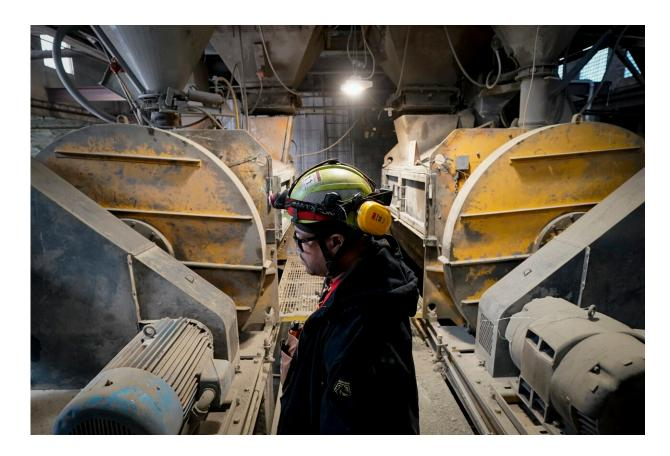
A worker stands beside the mixing machines at the start of a production line creating concrete blocks designed with liquid carbon dioxide as an ingredient at the Glenwood Mason Supply Company, Tuesday, April 18, 2023, in the Brooklyn borough of New York. New York is forcing buildings to clean up, and several are experimenting with capturing carbon dioxide, cooling it into a liquid and mixing it into concrete where it turns into a mineral. Credit: AP Photo/John Minchillo
