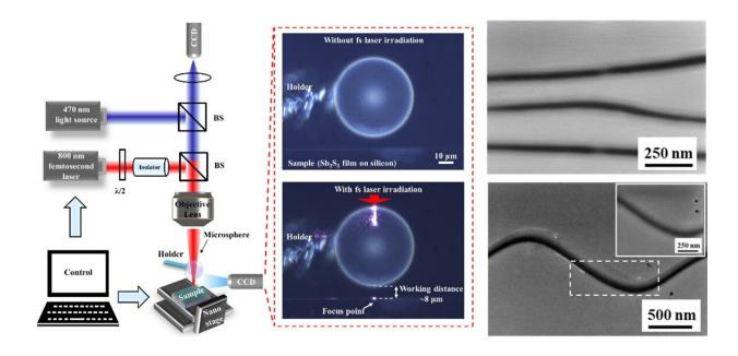
Fig. 1. Experimental setup of non-contact microsphere femtosecond laser irradiation and the fabricated nano-structures. Credit: Compuscript Ltd
