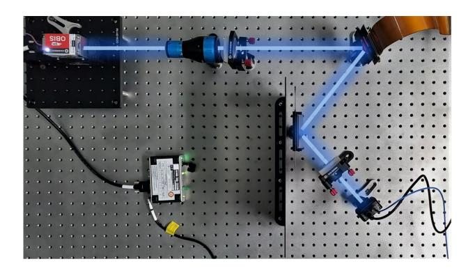
Researchers have developed a new high-speed way to detect the location, size and category of multiple objects without acquiring images or requiring complex scene reconstruction. The proof-of-concept setup for image-free single-pixel object detection (SPOD) is shown. Credit: Lintao Peng, Beijing Institute of Technology
