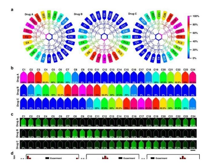
Generation of microfluidic drug concentration gradient under different flow conditions. (a) Simulation imaging of the generation process of the drug concentration gradient in the device. Three inlets were filled with drug A, drug B, and drug C when the flow rate was 10  $\mu$ L/min. (b) Numerical simulation of drug concentration gradient formation in 24 microchambers. (c) Concentration gradients formed by fluorescence experiments in 24 microchambers. The
