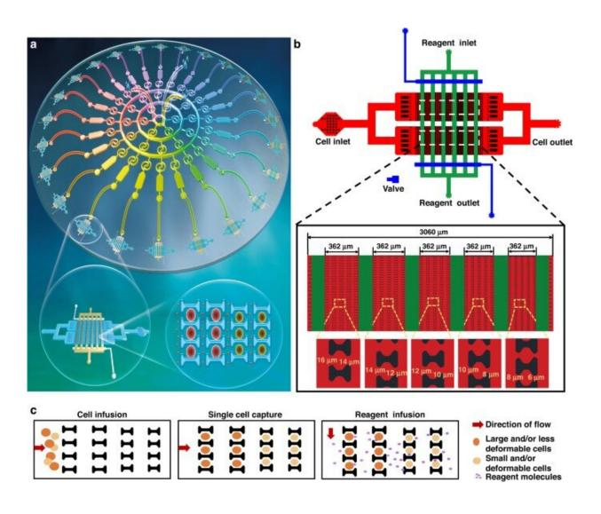
Drug screening at the single-cell level based on multiconcentration gradient construction and a single-cell capture device. (a) Schematic diagram of the integrated microfluidic device. (b) The detailed design of a single-cell capture device. The various channels are shown with different colors to visualize the
