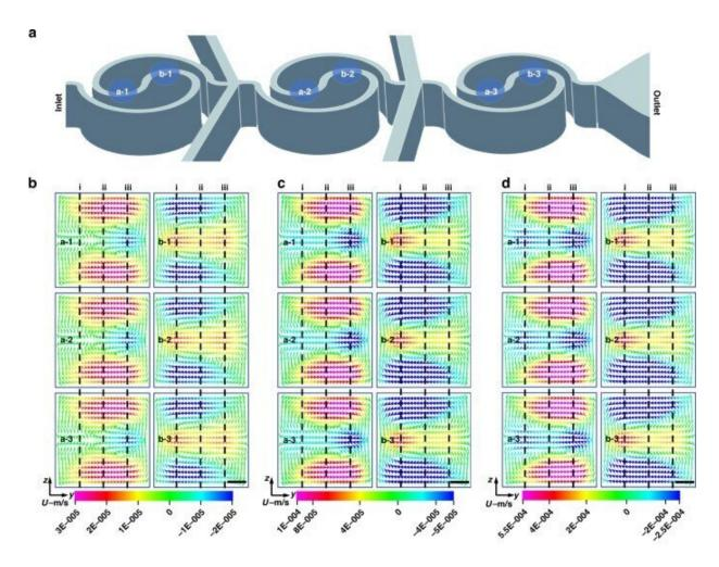
Tai Chi-spiral mixer–induced Dean flow. (a) Sketch diagram of spiral mixer channels. (b–d) Dean flow simulation at different positions in the channel when the flow rate was 10  $\mu$ L/min (b), 20  $\mu$ L/min (c), and 50  $\mu$ L/min (e). Scale bar: 10  $\mu$ m. e Quantitative analysis of cross-sectional Dean flow. The results are obtained at the positions shown in the dotted lines of Fig. 3b–d. Credit: *Microsystems & Nanoengineering* (2023). DOI: 10.1038/s41378-023-00516-0
