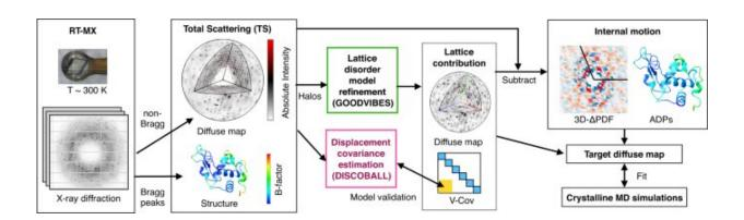
Workflow to measure and interpret protein correlated motion using X-ray crystallography. Credit: *Nature Communications* (2023). DOI: 10.1038/s41467-023-36734-3
