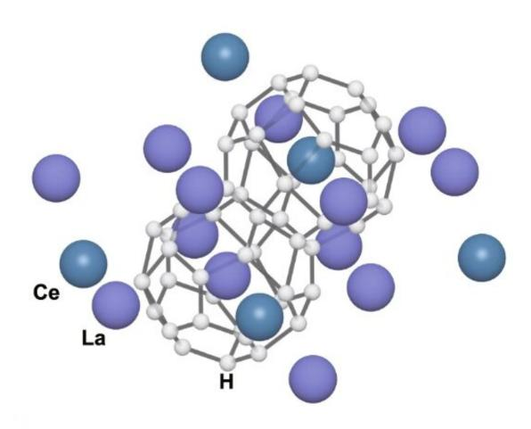
The structure model of the  $P6_3/mmc$ -(La,Ce) $H_{9-10}$ . Credit: *Nature Communications* (2023). DOI: 10.1038/s41467-023-38254-6
