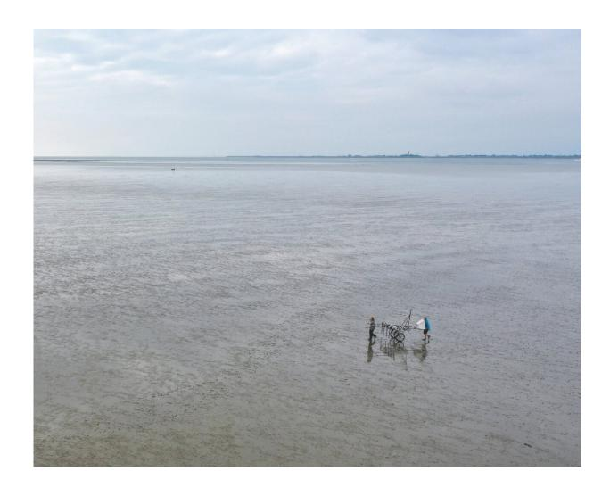
A lightweight survey vehicle provides large-scale magnetic mapping of cultural traces hidden beneath the present-day tidal flat surface. Credit: Dirk Bienen-Scholt
