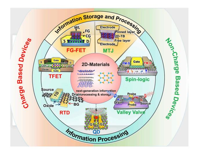
Illo caption: An array of charge-based and non-charge-based devices built with 2D materials may enable next-generation information processing and storage technologies. Four of the most promising devices — the spin-FET and the TFET (both for processing) as well as the FG-FET and the MTJ (both for storage) —
