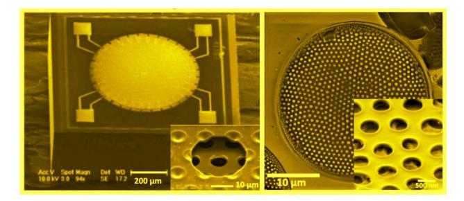
Image. MEMS microphone (left) and diatom (right) structure. Nature created an incredibly efficient structure, which is reminiscent of the manmade microphone membrane. Credit: Julijana Cvjetinovic/*Scientific Reports*
