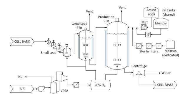
Fed-batch ACBM production system utilized in this LCA of ACBM. Credit: *bioRxiv* (2023). DOI: 10.1101/2023.04.21.537778
