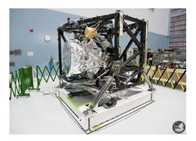
JWST's Mid-Infrared Instrument (MIRI is shown here, wrapped in its aluminized thermal shield while being integrated into the JWST Integrated Science Instrument Module (ISIM). Credit: NASA/Goddard Space Flight Center/Chris Gunn
