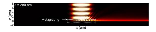
Visualization of light incident on a metagrating and its conversion into unidirectional SPPs. (Simulation). Credit: POSTECH
