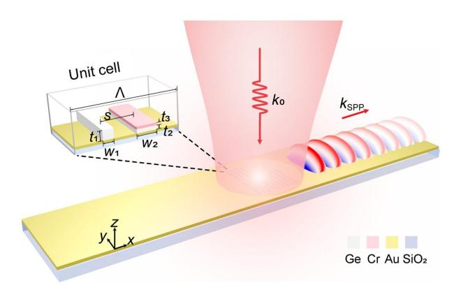
Schematic diagram of a metagrid that converts normally incident light into unidirectional SPPs. The unit cell of the metagrating consists of two different nanostructures and induces tailored optical losses. Credit: POSTECH
