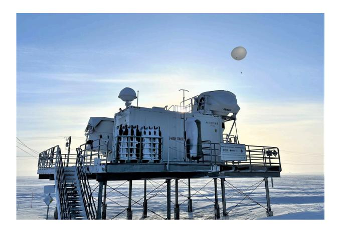
A hydrogen-filled weather balloon launches automatically from a Department of Energy atmospheric measurement facility in Utqiaġvik, formerly known as Barrow. About three years ago, Sandia National Laboratories switched from launching helium-filled balloons to launching hydrogen-filled balloons to reduce costs and carbon emissions. Credit: Ben Bishop/Sandia National Laboratories
