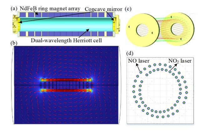
Single-cavity, dual-optical path gas cell; Magnetic field intensity distribution of NdFeB ring magnet array. Credit: Cao Yuan
