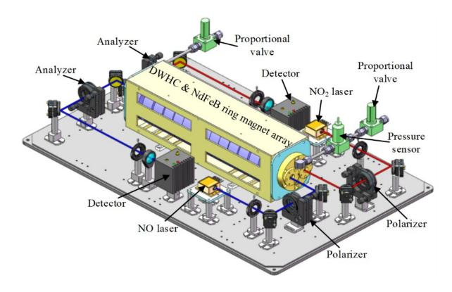
Optical layout of the FRS NO<sub>x</sub> sensor. Credit: Cao Yuan
