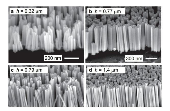
SEM images of specimens in this study taken from a tilt angle of 45°. Images in the left column portray the specimen set grown without a buffer layer (Set A), and the right column portrays the specimen set grown with an AlN buffer layer (Set B). Run numbers are (a) D420, (b) D469, (c) D421, (d) D480, (e) D422, (f) D443, (g) D423, (h) D481. Credit: *Advanced Materials* (2023). DOI: 10.1002/adma.202209779
