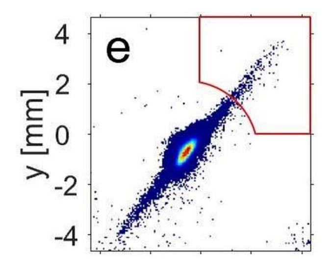
Electrons being scattered out of the main bunch using a intense laser pulse to measure the electron bunch length, Credit: de Raadt, Franssen & Luiten. (*PRL*, 2023)
