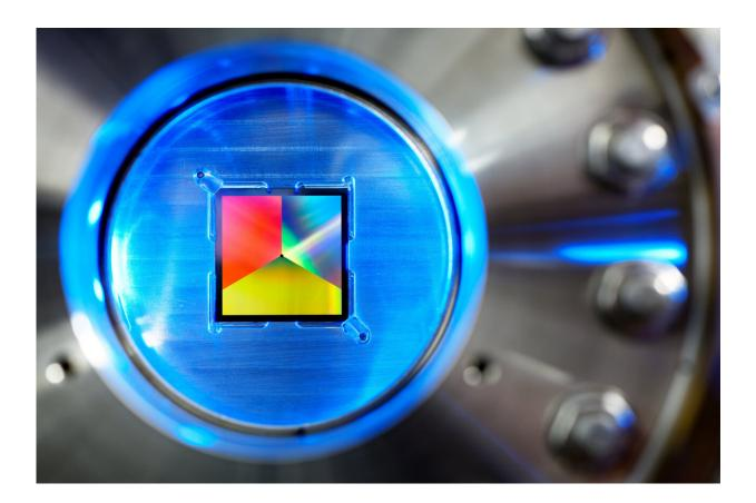
The grating at the heart of the ultra-cold electron source used for laser cooling. Credit: TU/e, Bart van Overbeeke.
