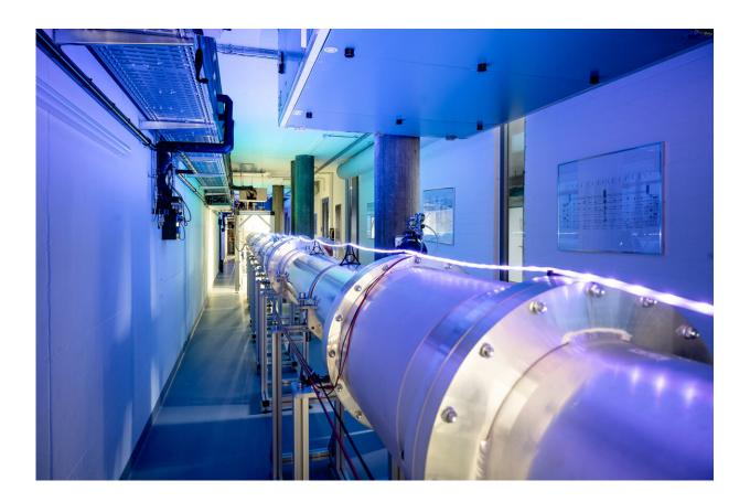
Partial section of the 30-meter-long quantum connection between two superconducting circuits. The vacuum tube (center) contains a microwave waveguide that is cooled to around  $-273^{\circ}$ C and connects the two quantum circuits. Credit: ETH Zurich / Daniel Winkler
