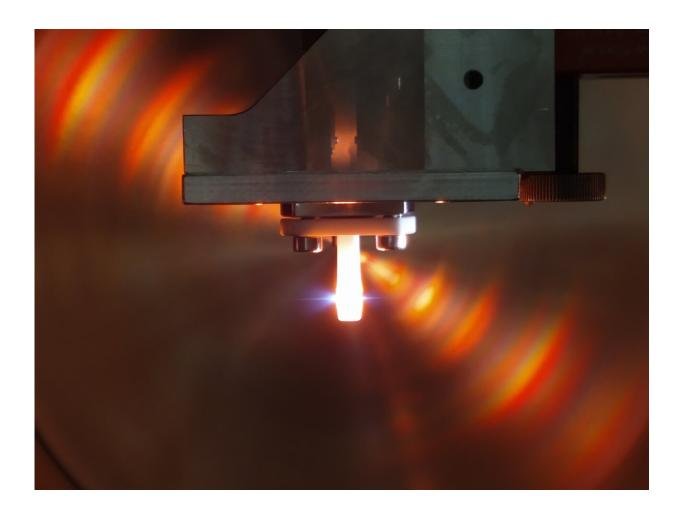
Fig. 1: Photo of the gas cell for high harmonic generation of extremely shortwavelength ultraviolet attosecond pulses. Credit: Max Hartmann, MPI für Kernphysik
